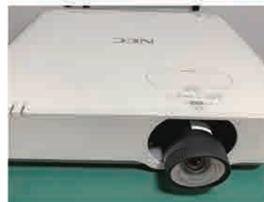
乐都0.7:1短焦, 安装到NEC NP-P605UL上, 凸出投影机机身5.5厘米。 LEDU 0.7:1 Short-throw Lens Installed on NEC NP-P605UL, protrude 5.5cm from the projector body.
