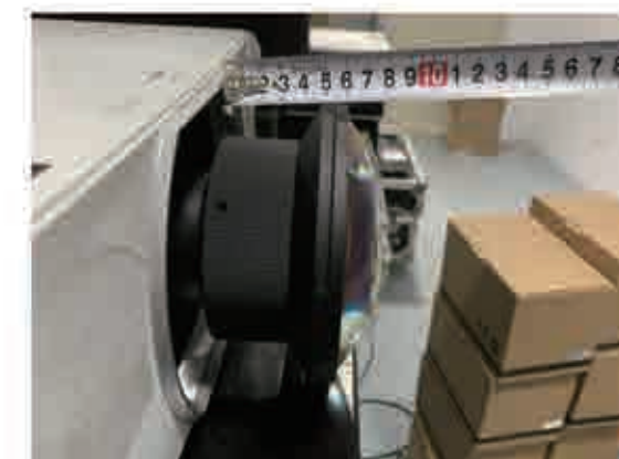
乐都0.5:1超短焦, 安装到NEC NP-PA803U上, 凸出投影机机身7.8厘米。 LEDU 0.5:1 Ultra Short-throw Lens Installed on NEC NP-PA803U, protrude 7.8cm from the projector body.
