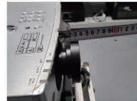
乐都0.6:1短焦, 安装到Panasonic(松下)PT-VMZ50上, 凸出投影机机身3.3厘米。 LEDU 0.6:1 Short-throw Lens Installed on Panasonic PT-VMZ50, protrude 3.3cm from the projector body.
