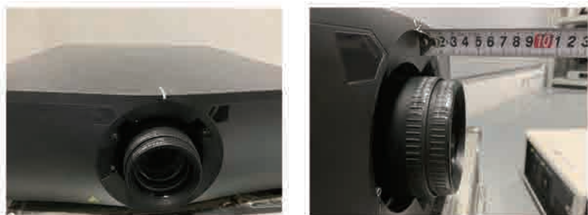
乐都3.5-6.3:1电动长焦, 安装到Christie(科视)D20WU-HS上, 凸出投影机机身4厘米。 LEDU3.5-6.3:1 Electric Zoom Lens Installed on Christie D20WU-HS, protrude 4cm from the projector body.
